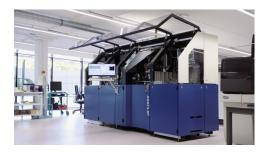
Fig. 1. ITEC's ADAT3-XF die bonder platform. [11]
